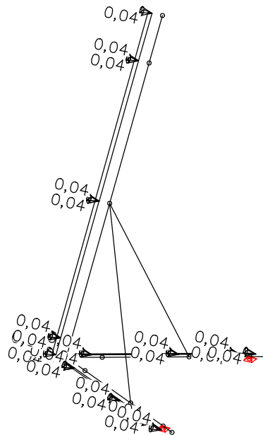
LC 12: Load, Wind on trusses x
