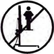
**3.1** - The TE-076 is a machine designed to elevate loads upwards in a vertical direction, It should NEVER be used as a platform to elevate people.
