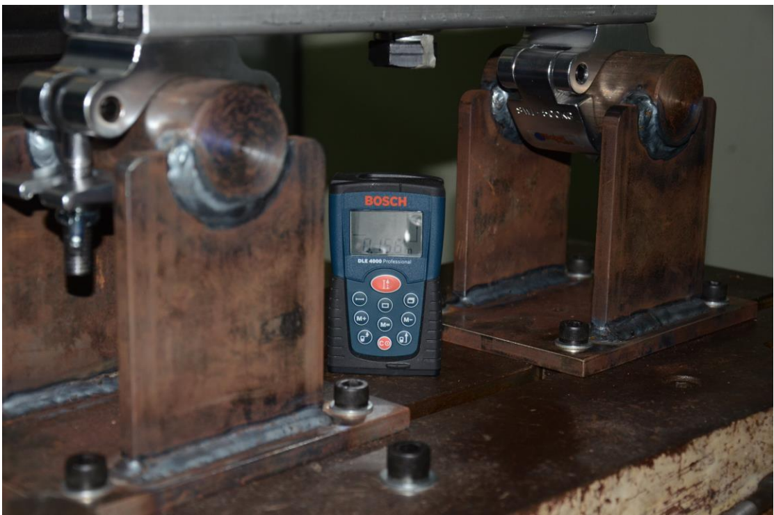
Distance is 0.157m after loaded deformation of the specimen at five minutes
