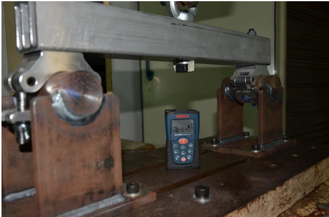
Distance is 0.164m after loaded deformation of the specimen at five minutes
