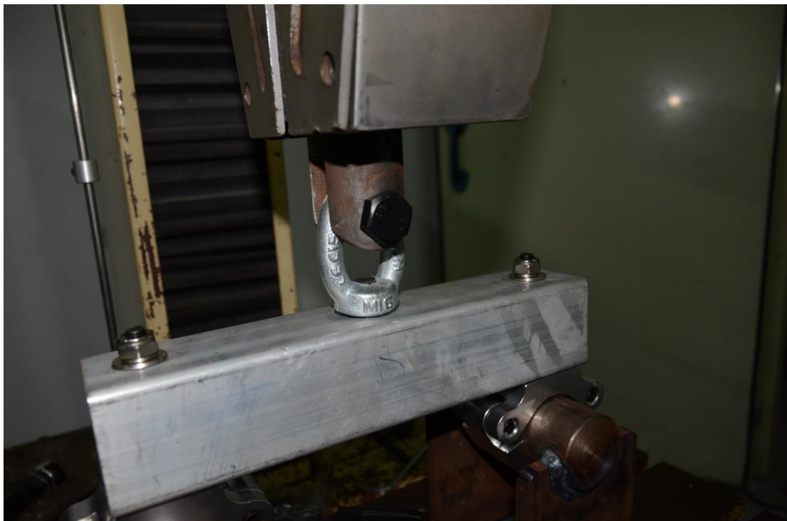
The eye bolt are obviously elongated, others No obvious deformation
