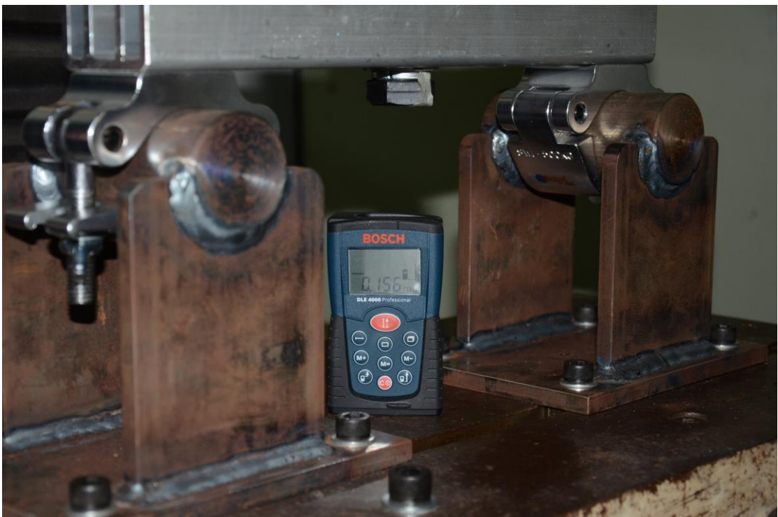
Distance is 0.156m Unload the specimen
