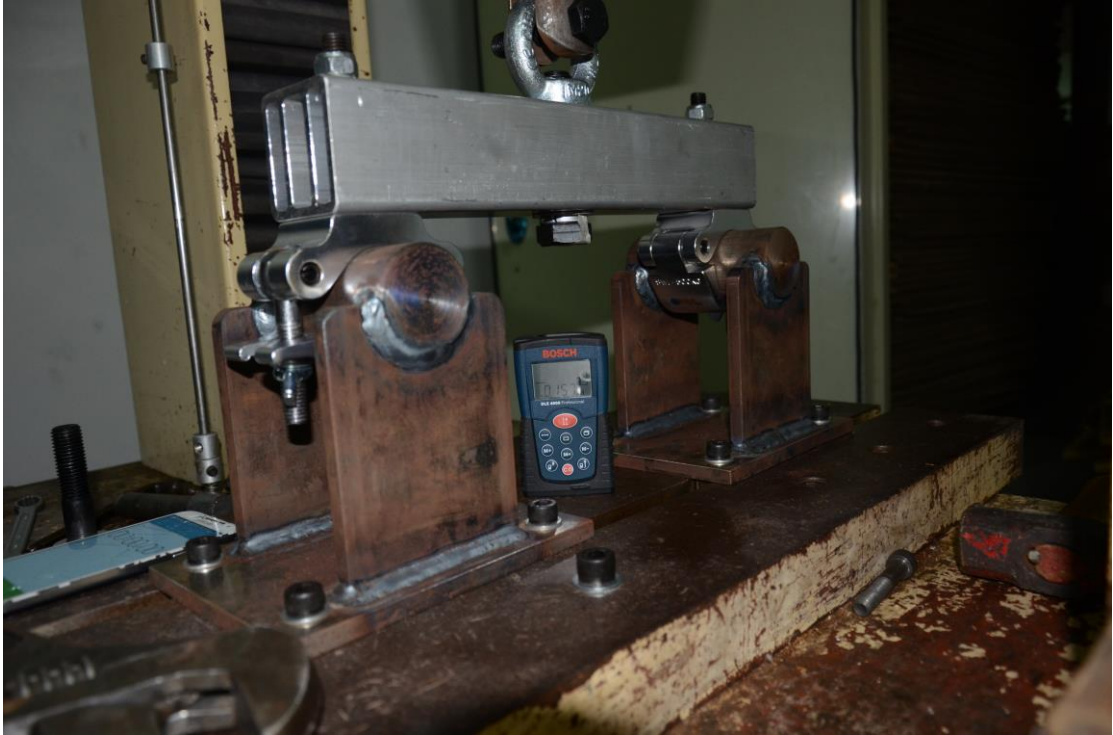
Distance is 0.157m after loaded deformation of the specimen at five minutes
