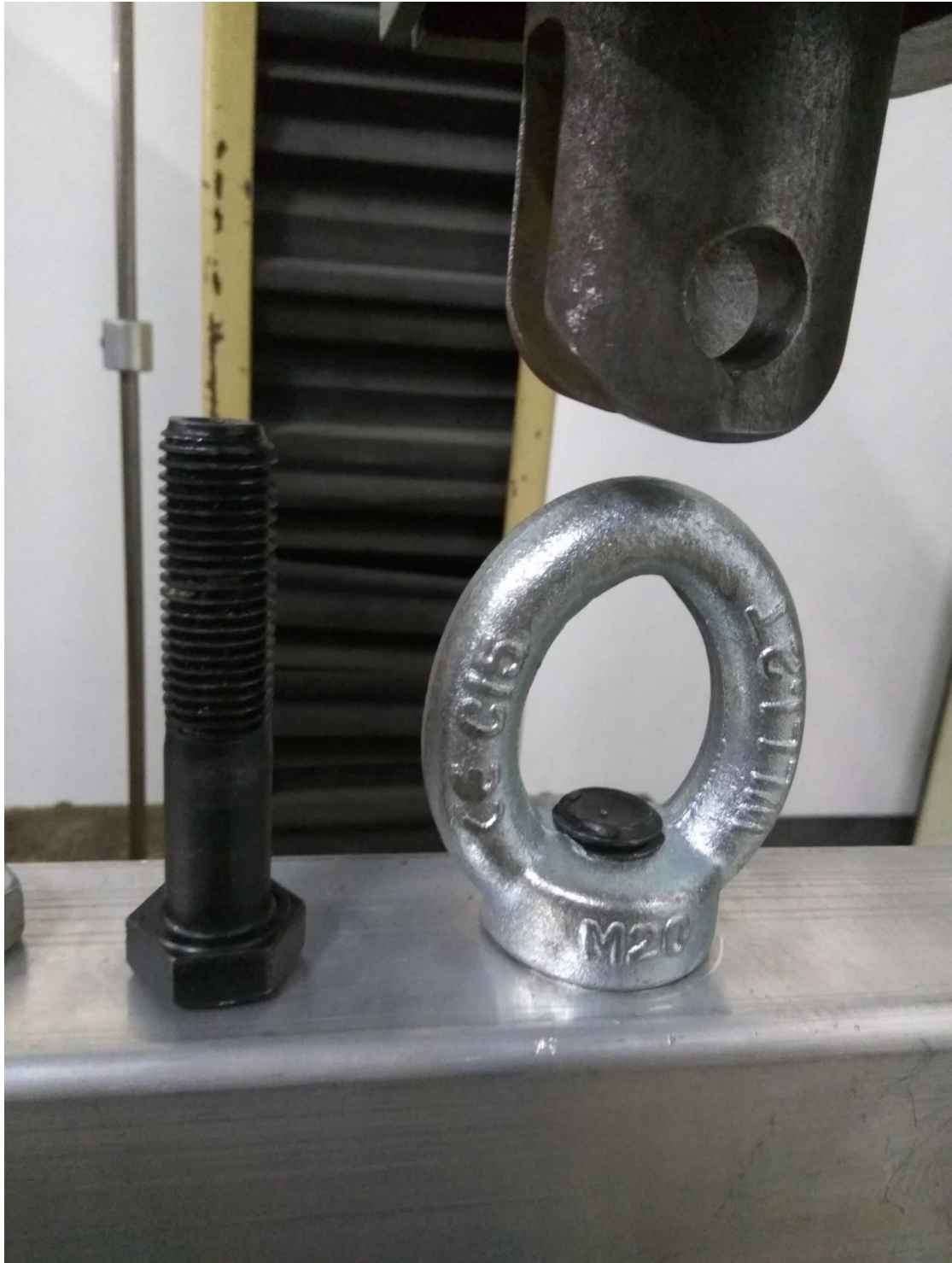
The eye bolt are obviously elongated, others No obvious deformation
