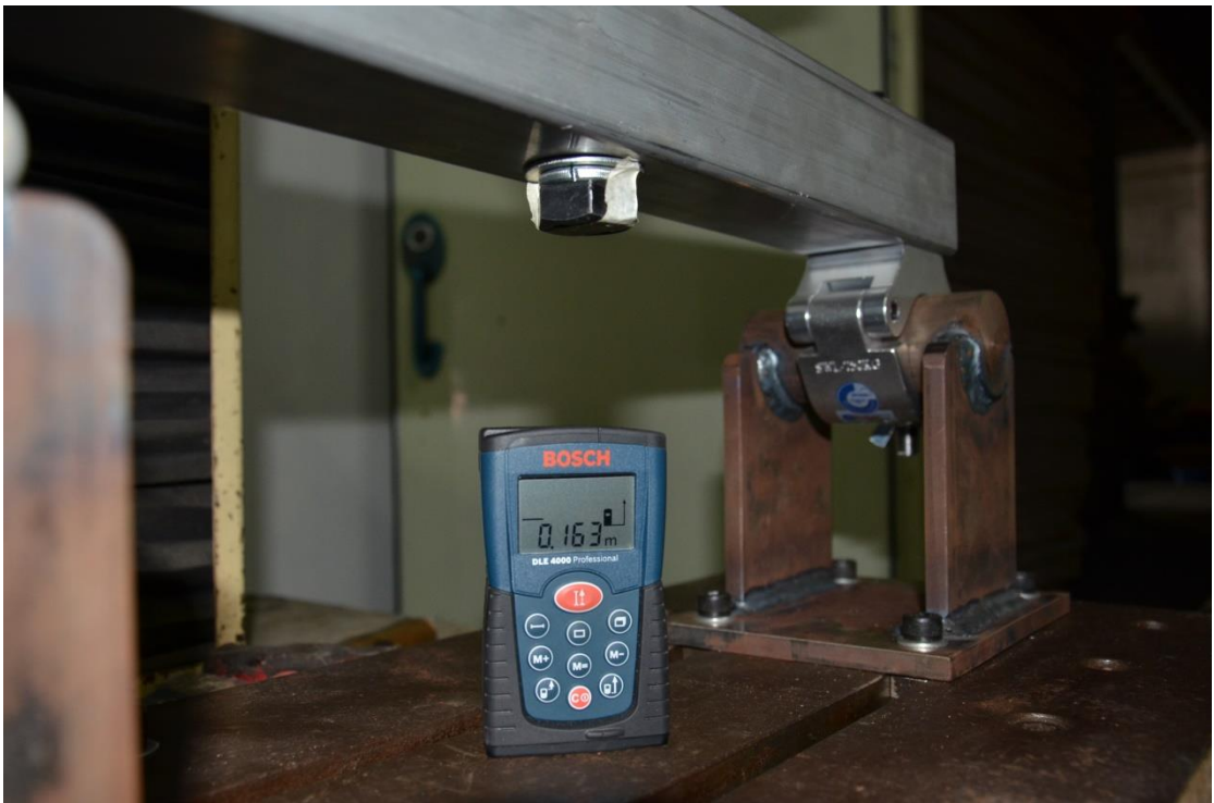
Before apply a test load, distance between plate and screw is 0.163m
