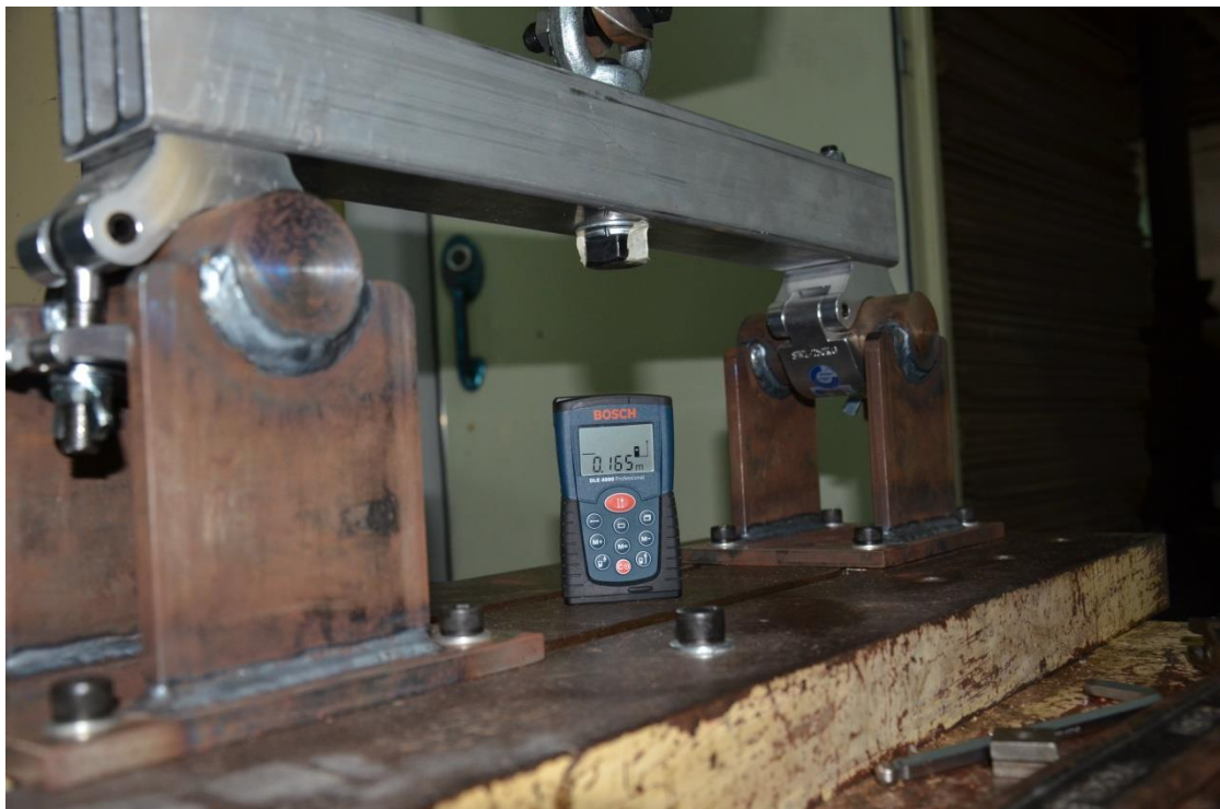
Distance is 0.165m after loaded deformation of the specimen at five minutes
