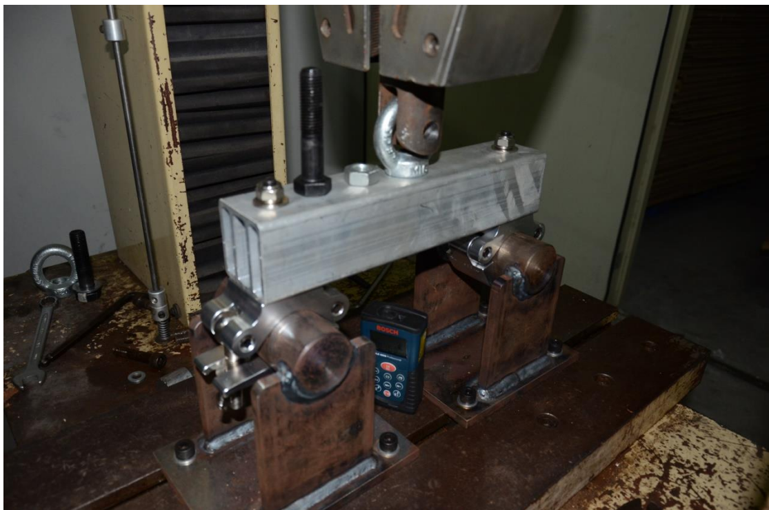
Distance is 0.163m Unload the specimen
