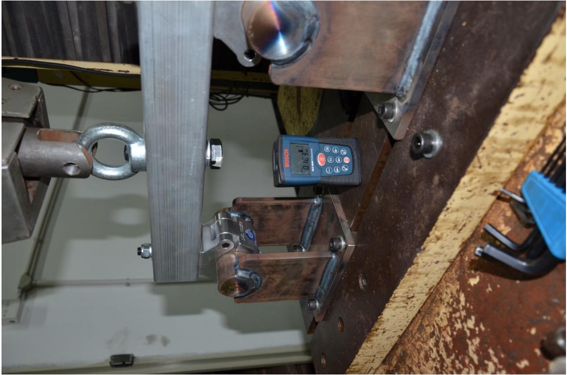
Distance is 0.163m Unload the specimen
