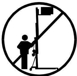
**3.10** - NEVER move the lift whilst it is carrying a load. It is not advisable to carry out any type of movement even small positional adjustments.
