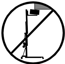
**3.8** - Take care with all obstacles above the lift and its extension zone such as cornices, balconies, and luminous signboards. It is very important to avoid the presence of all types of cables below the extended lift.
