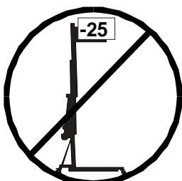
**3.14** - The minimum load to avoid problems regarding the breaking mechanism is 25KG. Without this load the brake will not work.
