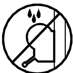
**3.15** - Do not grease or lubricate the winch's breaking mechanism. The brake disks have been greased with a special heat and pressure resistant solution. Other products should not be used to avoid negative effects regarding the braking mechanism.
