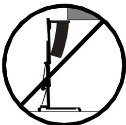
**3.8** – Be careful of any high, obstructions such as balconies, signs etc. It is important to avoid the presence of cables beneath the working position of the lift.
