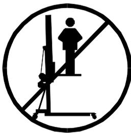
**3.1** – The TL-A320 is designed for lifting Line Array and should never be used for elevating persons.
