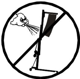
**3.6** – If there is excessive wind, place the lift on firm ground and attach slings to add stability. Never attach a sling to a vehicle or any other element than can move.
