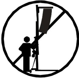
**3.10** – Never try to move the lift once the load is raised.
