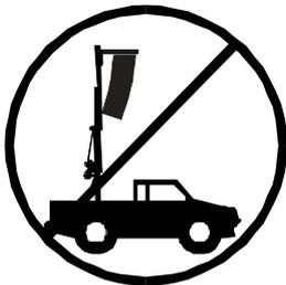
**3.11** – Never use the lift on a mobile surface or on any vehicle.
