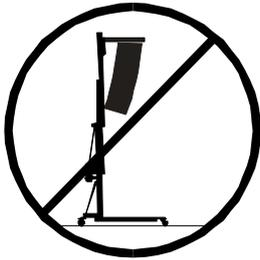
**3.4** – Never elevate the Line Array before checking it is correctly attached to the lift.
