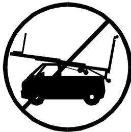
**3.16** – All profiles must be lowered before the lift is transported.
