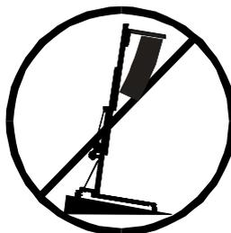
**3.2** – Only situate the lift on hard, flat surfaces checking that it is in a vertical position with the spirit level (**F**) included. If necessary, adjust with support stabilisers (**Q**) by turning the handle (**H**). Do not use any other materials to balance the lift.
