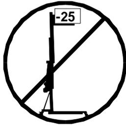
**3.14** – The minimum load for the brake functioning in the winch is 25kg. Without this weight the brake will not function.
