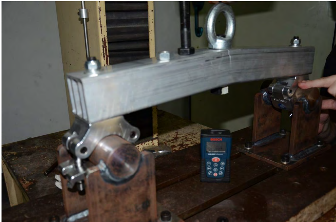
The eye bolt elongated, and the tube break
