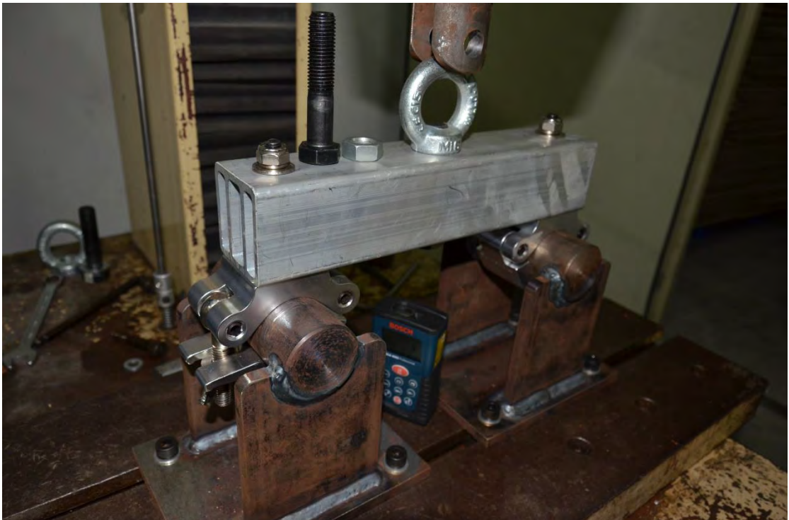
Distance is 0.163m after loaded deformation of the specimen at five minutes
