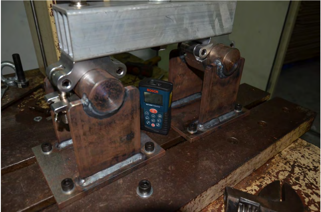
Distance is 0.163m after loaded deformation of the specimen at five minutes
