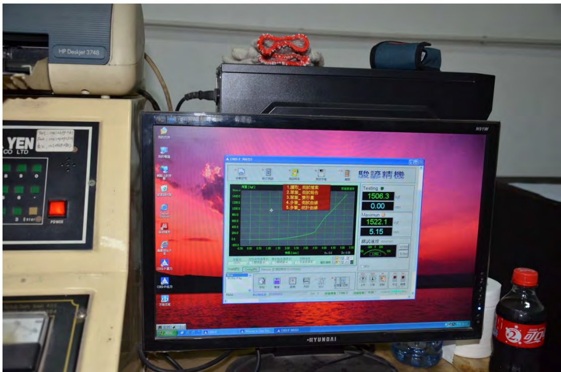
Apply a test load of 1500kg
