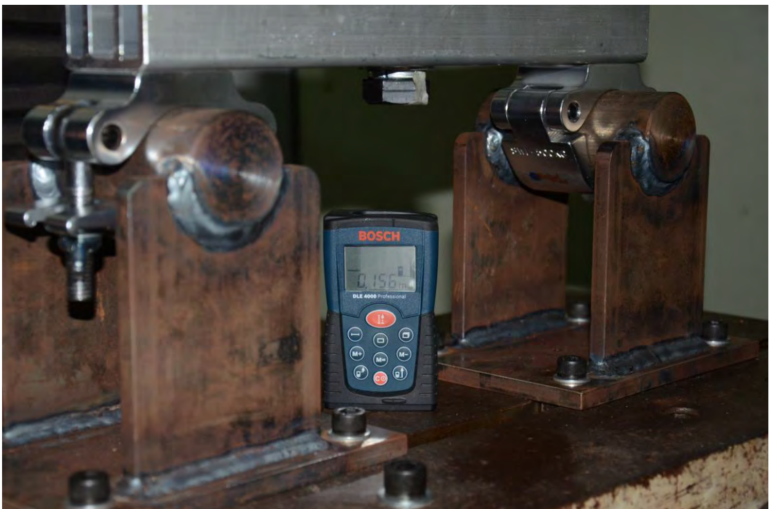
Distance is 0.156m Unload the specimen
