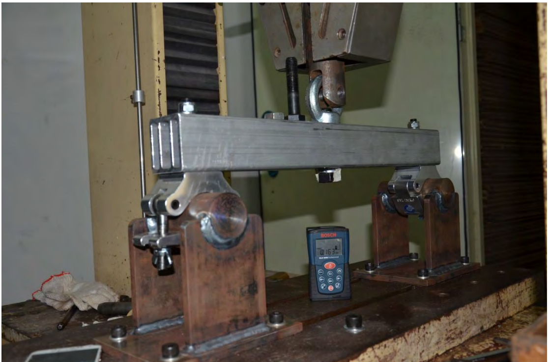
Distance is 0.163m Unload the specimen
