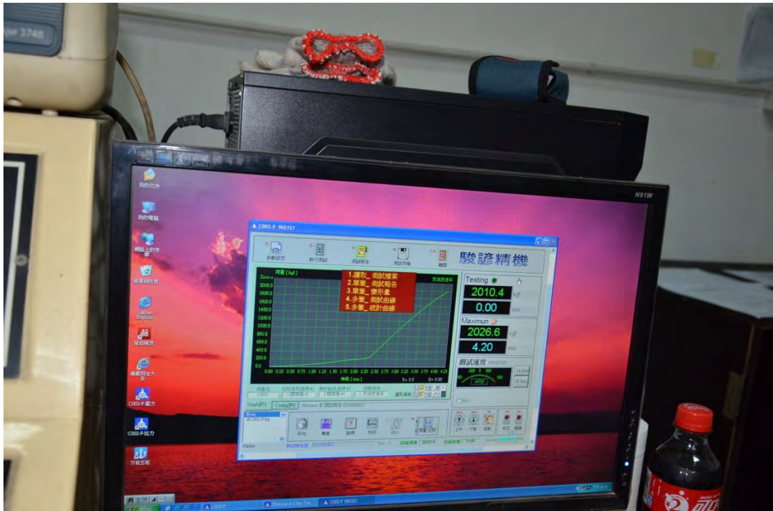
Apply a test load of 2000kg
