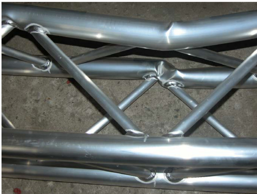
Figure 10 Local Bearing Failure of Chord of Global Truss F34 Square Truss
