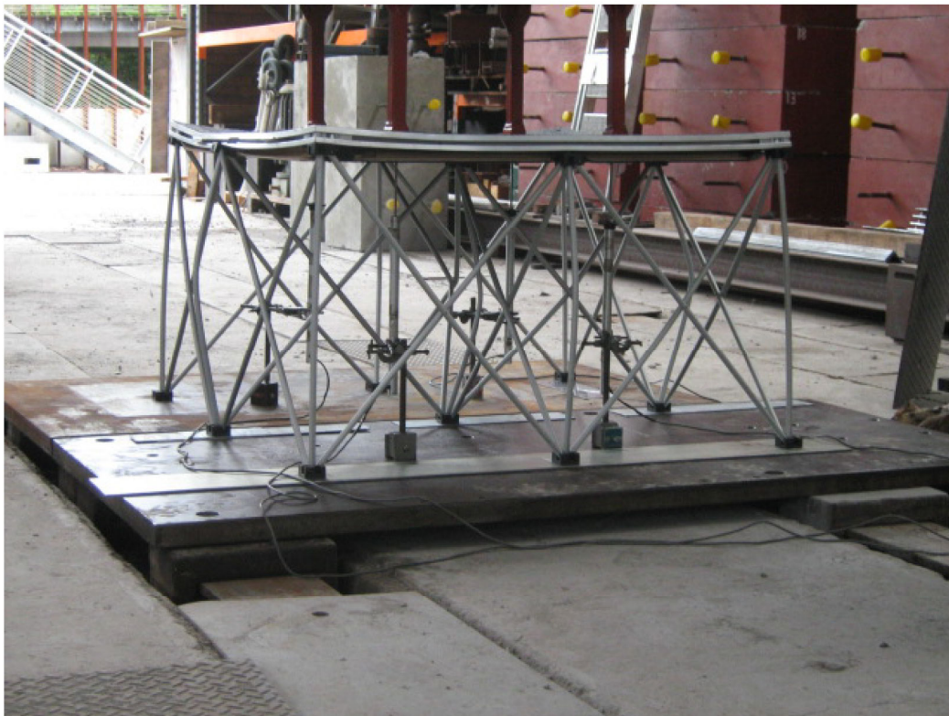
Figure 8 Concertina Stage During Testing
