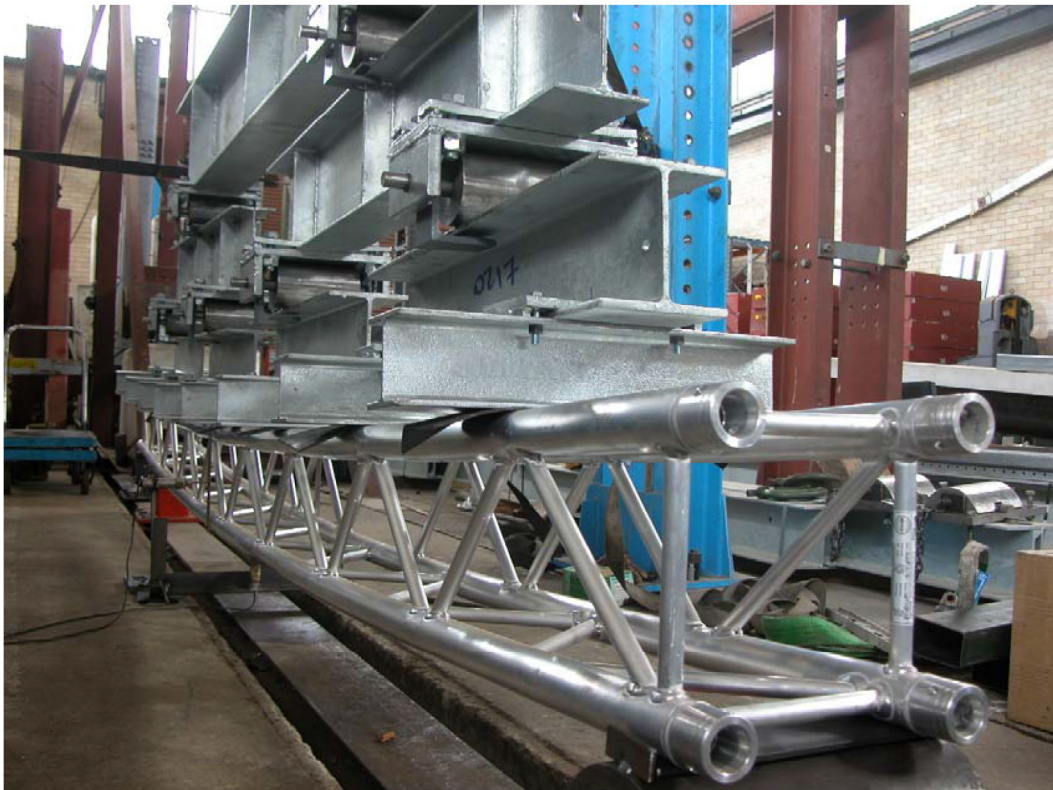
Figure 7 Global Truss F34 Square Truss During Testing
