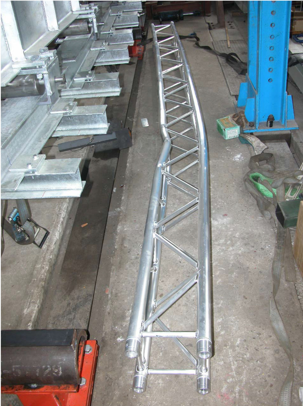
Figure 11 Member Buckling Failure of Global Truss F34 Square Truss
