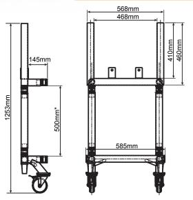
\*Height can easily be adjusted by increasing/decreasing truss spacers or F01 Tube lengths
