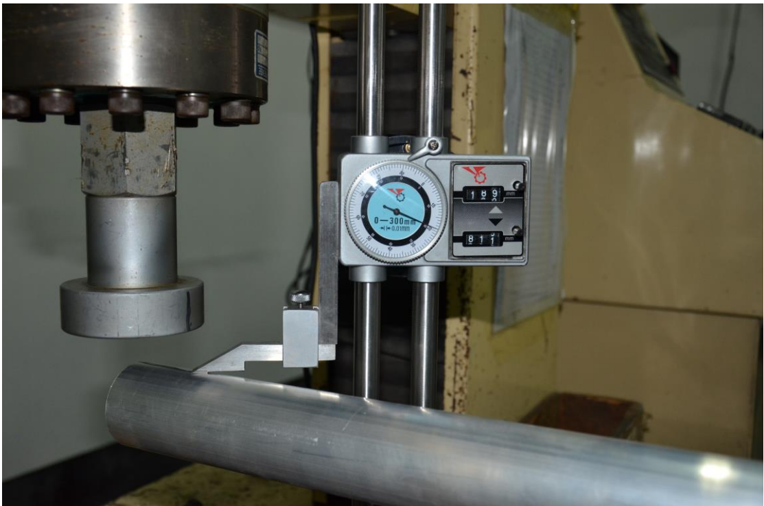
Distance is 189.2mm Unload the specimen
