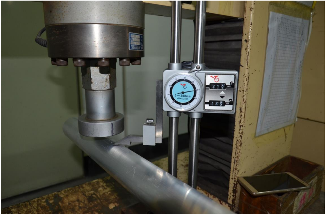
Distance is 210.5mm Unload the specimen
