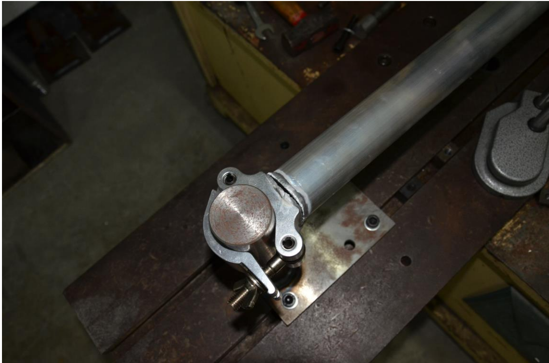
The tube fracture at weld, others No obvious deformation
