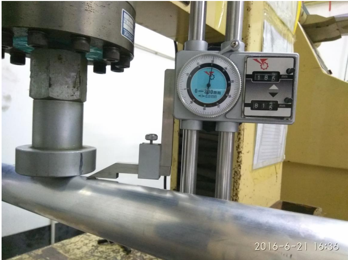
Distance is 184.3mm after loaded deformation of the specimen at five minutes
