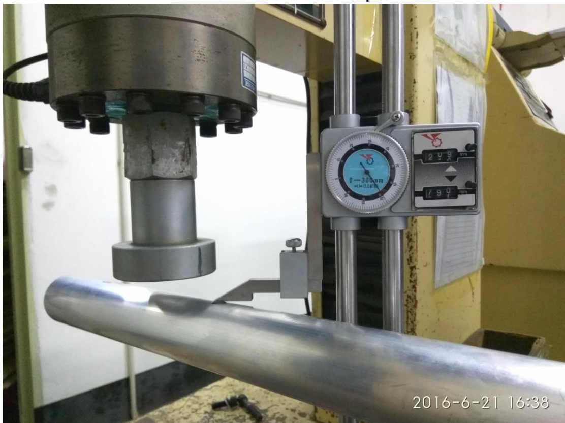
Distance is 209.7mm Unload the specimen
