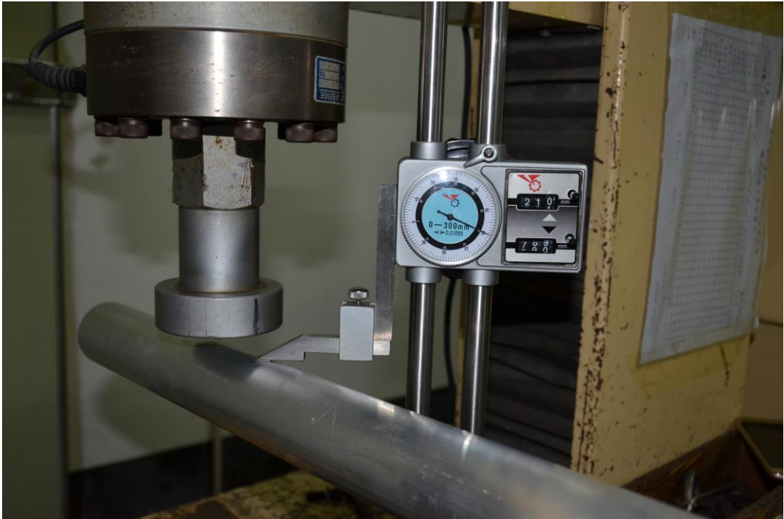
Distance is 210.6mm Unload the specimen
