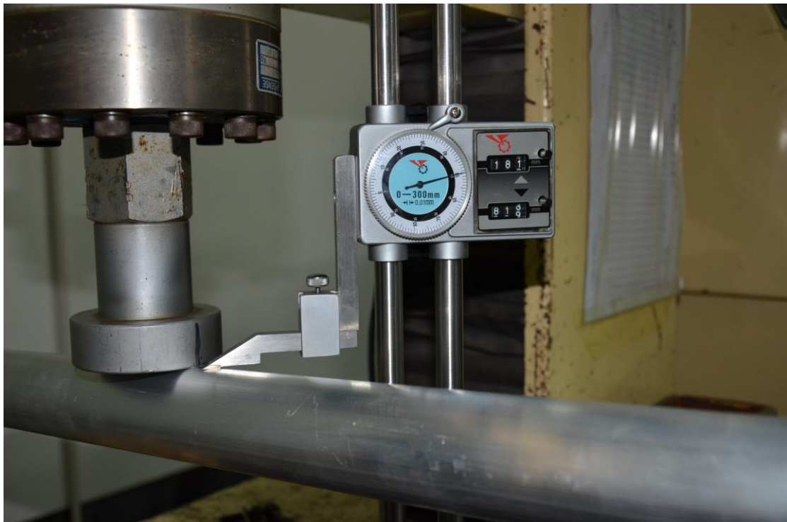
Distance is 181.5mm after loaded deformation of the specimen at five minutes
